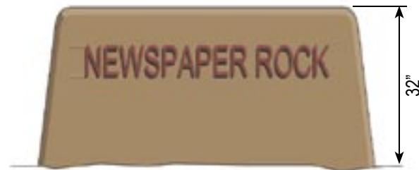
CMU sign with stucco finish with painted aluminum letters
