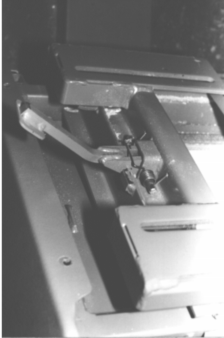
Figure B-10. Locking Mechanism Photograph, Mechanism in the Locked Position
