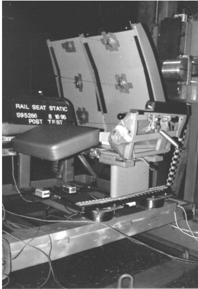
Figure 5-2. Head-Load Quasi-Static Test, Seat Pair Post-test Condition
