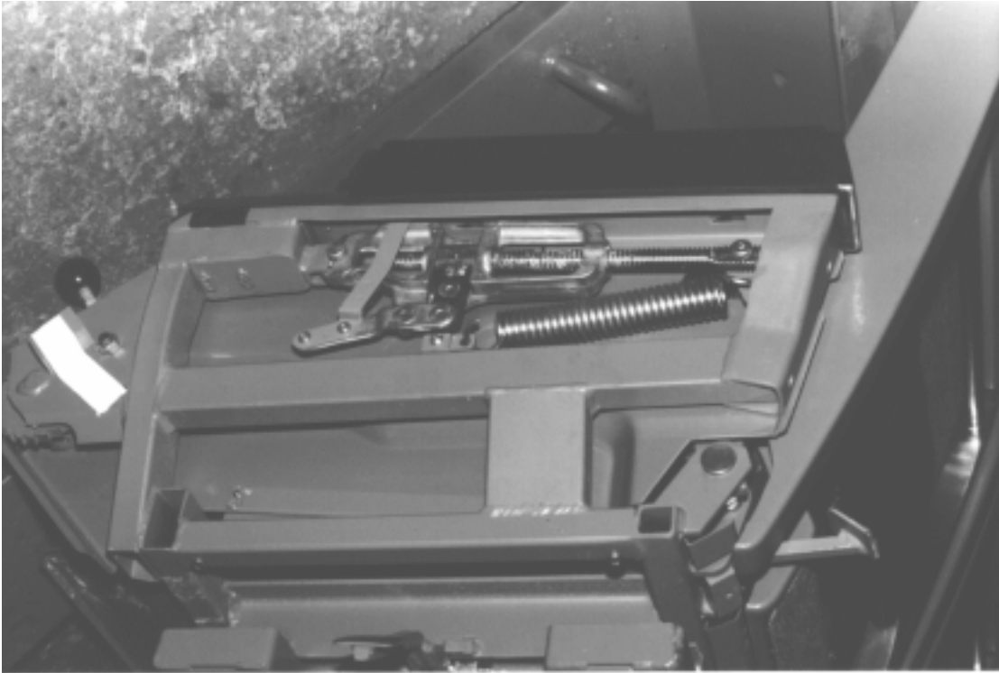
Figure B-12. Recline Mechanism Photograph
