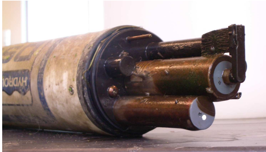
Figure 5. Biofouling on the Hydrolab DS5X data sonde after a two week deployment.
