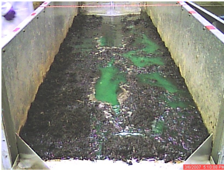
Figure 3: Erosion process on commercial erosion control compost
