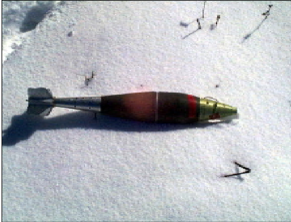
Figure 3. An 81-mm mortar round placed on its side on the surface of the snow.
