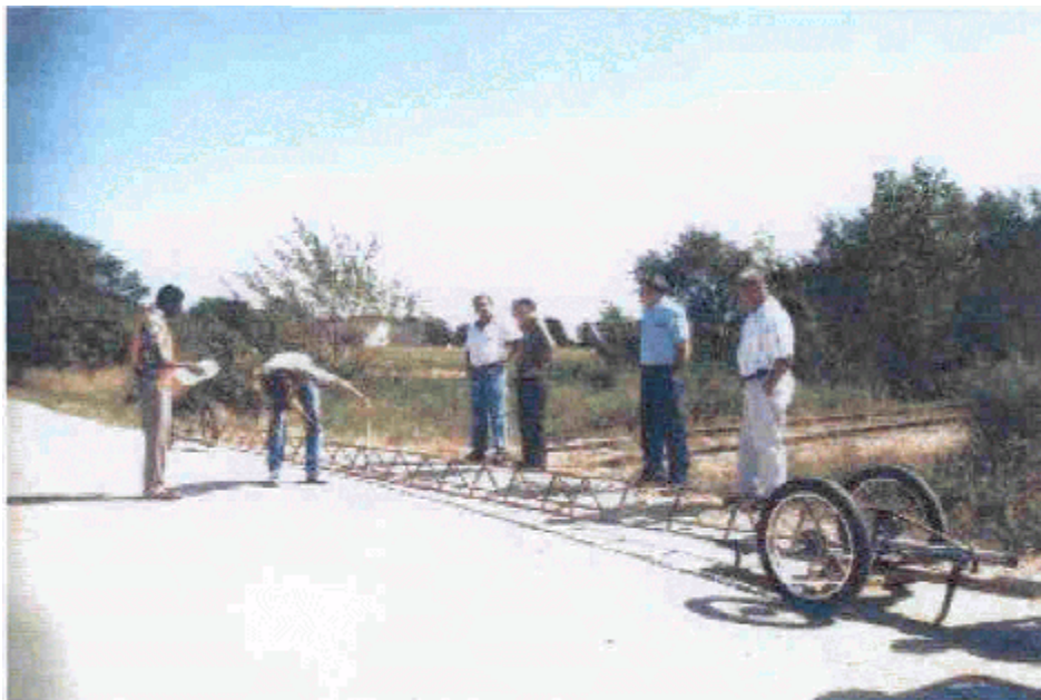
FIGURE 16: Taking Clearance Measurements from the Prototype Model
