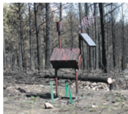
C. Precipitation gage used in burned area at Battle Creek Fire.
