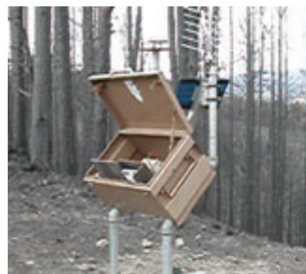
B. Precipitation gage used in burned area at Grizzly Gulch Fire.
