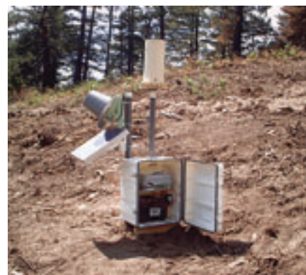
A. Precipitation gage (instrument detail) used in burned area at Missionary Ridge Complex Fire.
