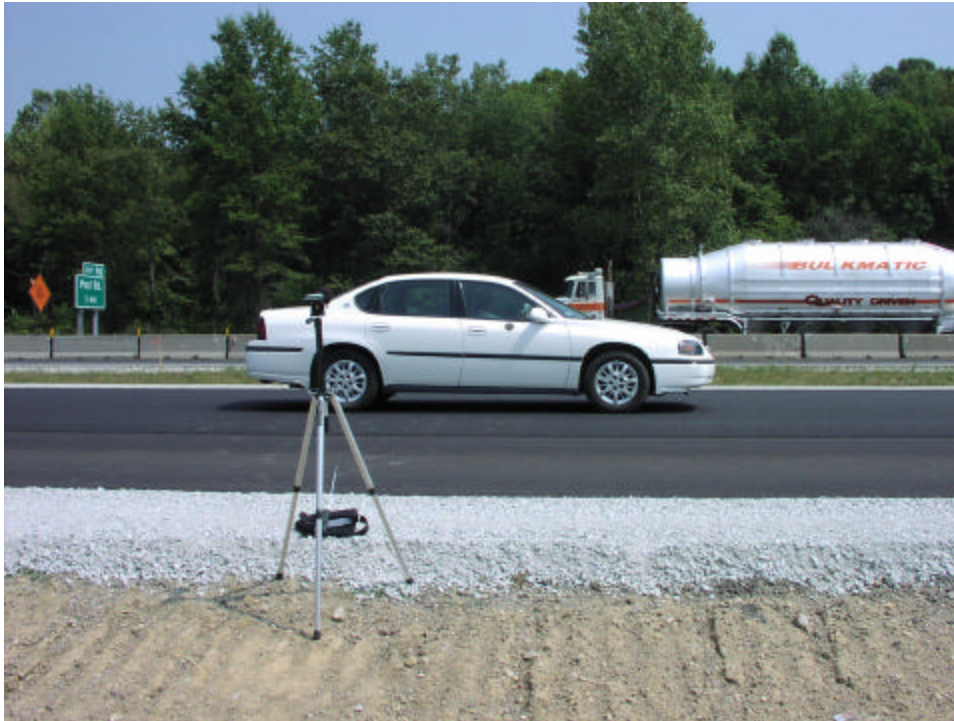
Figure 8. Pass-By Measurement Site (I74) and Microphone Setup
