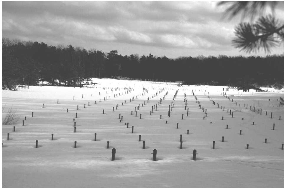
USGS Toxic Substances Hydrology Research Site, Falmouth, Cape Cod, Massachusetts--array of wells and multi-level samplers used to investigate processes controlling the fate and transport of contaminants in ground water. (photo by D. R. LeBlanc)
