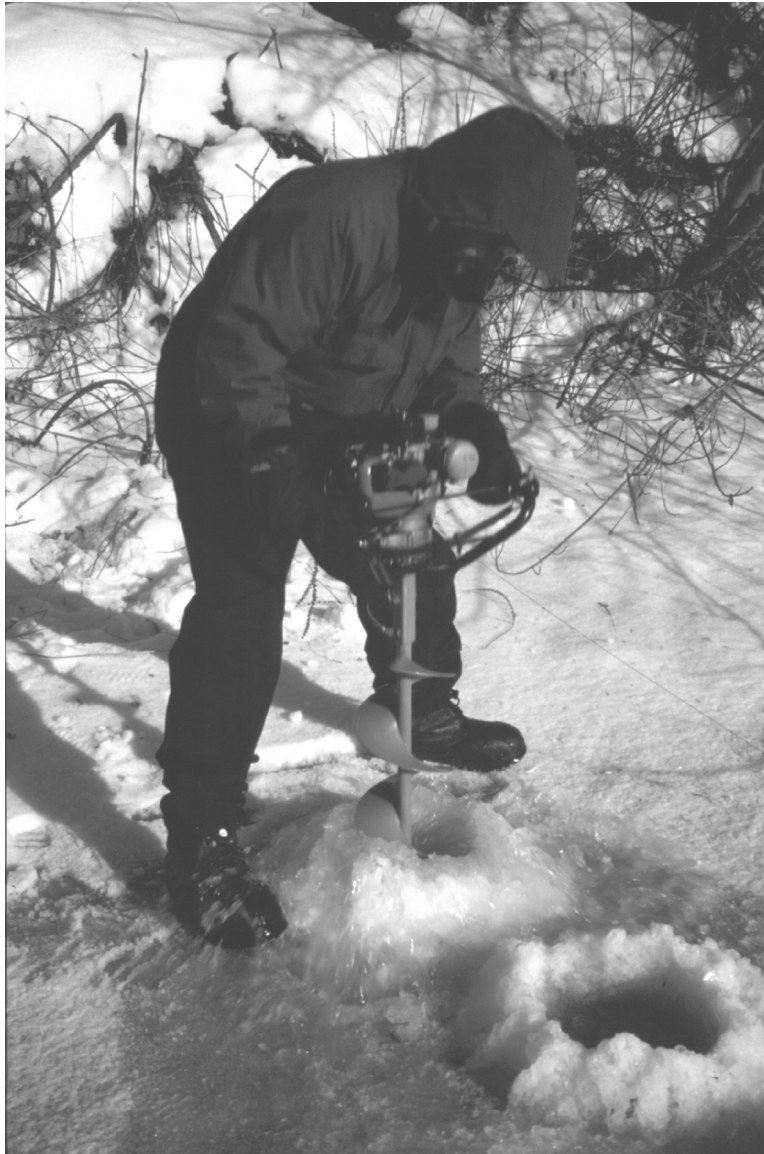
Hydrologic Technician Joe Zanca drilling holes for ice discharge measurement at Charles River at Medway, Massachusetts, February 1, 2000. (photo by L. Y. Comeau)
