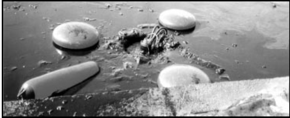
Skimmers, like the one pictured here, are used to collect spilled oil.
