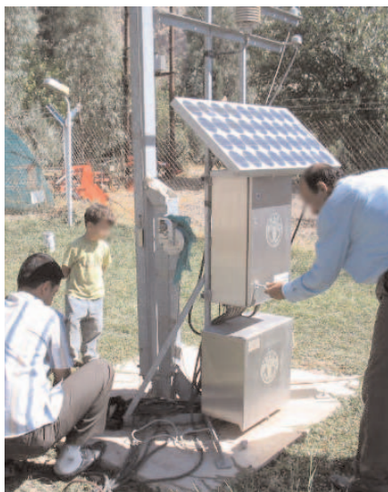
An automatic weather station with a solar collector which provides power in remote locations.
