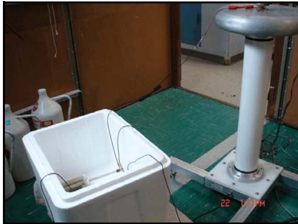
Fig. 2. Tape assembly in Styrofoam dewar, connected to voltage divider.
