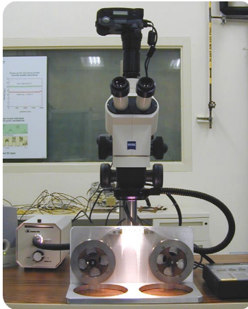
Fig. 1.6. Reel-to-reel optical examination system.
