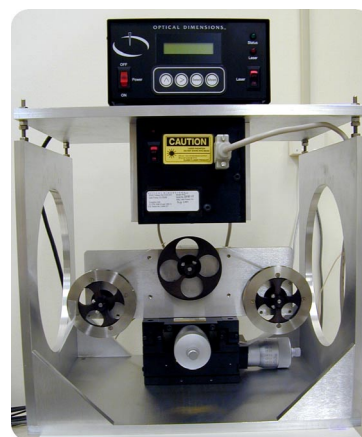
Fig. 1.4. Reel-to-reel surface roughness measurement system.
