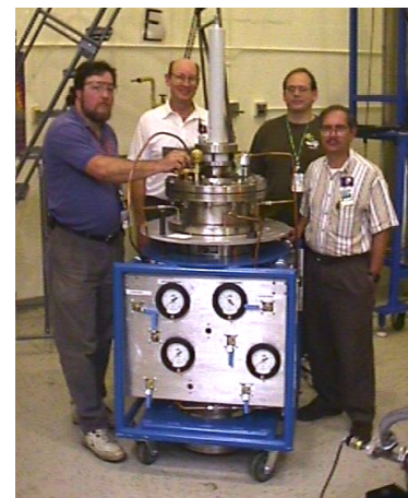
Fig. 2.37. Partial discharge and aging pressurized cryostat for short-length (2-ft) model cables. Partial-discharge pulses can be monitored on the ground side of the cable.
