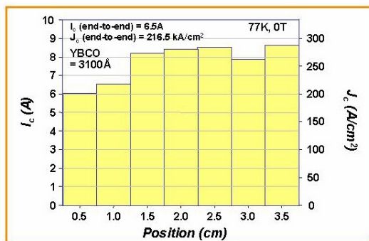
Fig. 1.59. J_c distribution of a 5-cm sample. Total voltage separation is 3.5 cm.
