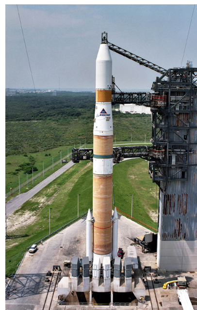
Boeing Delta IV (4-m fairing with 2 solid strap-on motors) at Cape Canaveral, FL
