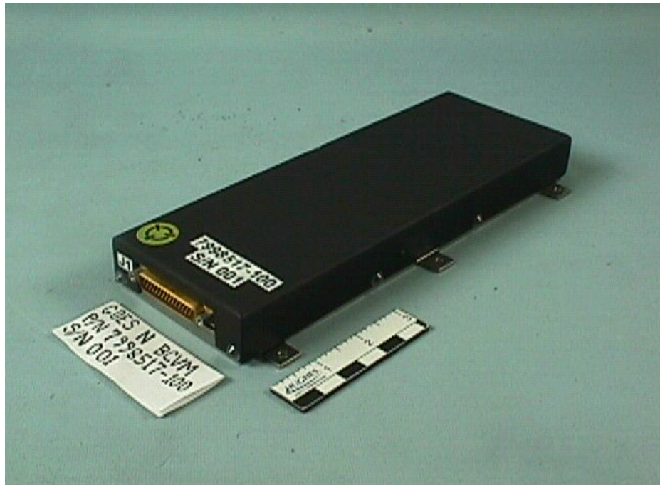
Figure 10-6. Battery Cell Voltage Monitor
