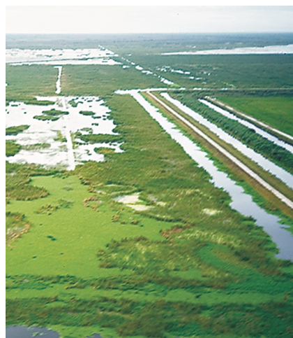
Canals and a levee separate constructed wetland from the agricultural area to the right.
