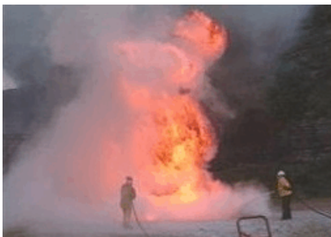
Figure 6.—Extinguishing a 400-ft 2 liquid fuel fire.
