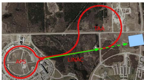
FIGURE C.1 The Proposed APS Energy Recovery Linac
