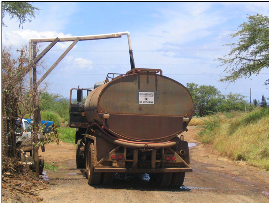
Maui County is the only county in Hawaii to consistently use recycled water for dust control.
