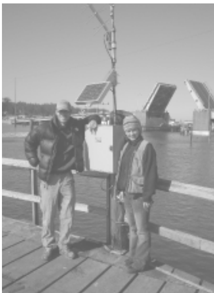
Ali and Adam with the SWMP real-time data transmitter that sends water quality data to two satellite arrays and from these the data are beamed to a NASA and a NOAA station where it is then sent to the CDMO (Centralized Data Management Office) and posted on the internet. Check it out at http://cdmo.baruch.sc.edu .
