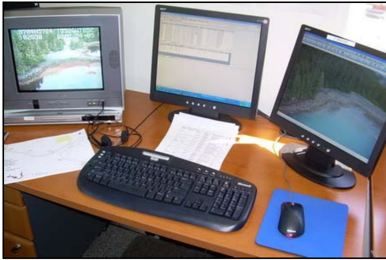
Figure 3.2. Photo of mapping station setup with DVD player (left), database window (center screen), and still photo viewer (right). Headphone facilitate audio use. Segmentation (paper) map is at left.
