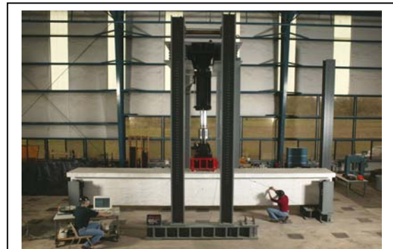
Testing the load-bearing capacity of a full-scale bridge beam at OSU's Hinsdale Wave Laboratory
