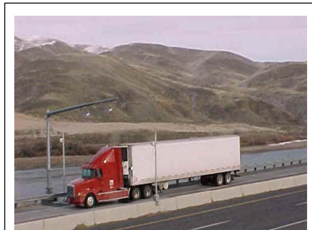
An 18-wheeler is weighed in motion, identified by its transponder, and signaled to pass the Farewell Bend Port of Entry.
