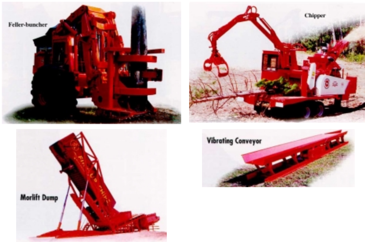
Fig. 6-3. Tree harvest and chipping equipment (Morbark Inc., 1998).
