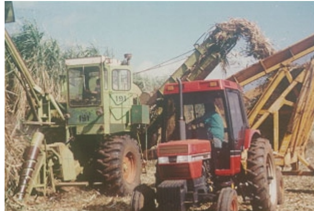
(b) Claas Model CCI400 sugarcane harvester transferring chopped banagrass into Vanguard Model V1248-2 tipper trailer (20 cubic yard capacity) for infield transporting/transloading.
