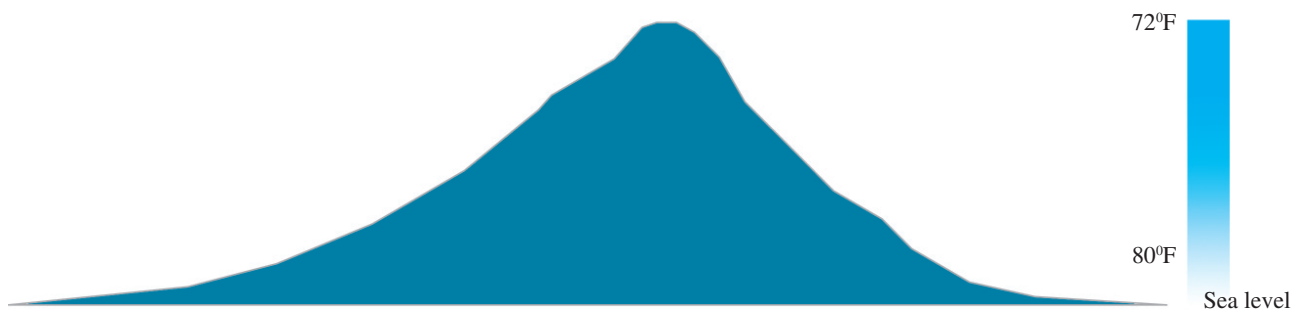
Fig. 4-1: Air Temperature Variation with Altitude. Air temperatures decrease about 3° F per thousand feet of rise above sea level.
