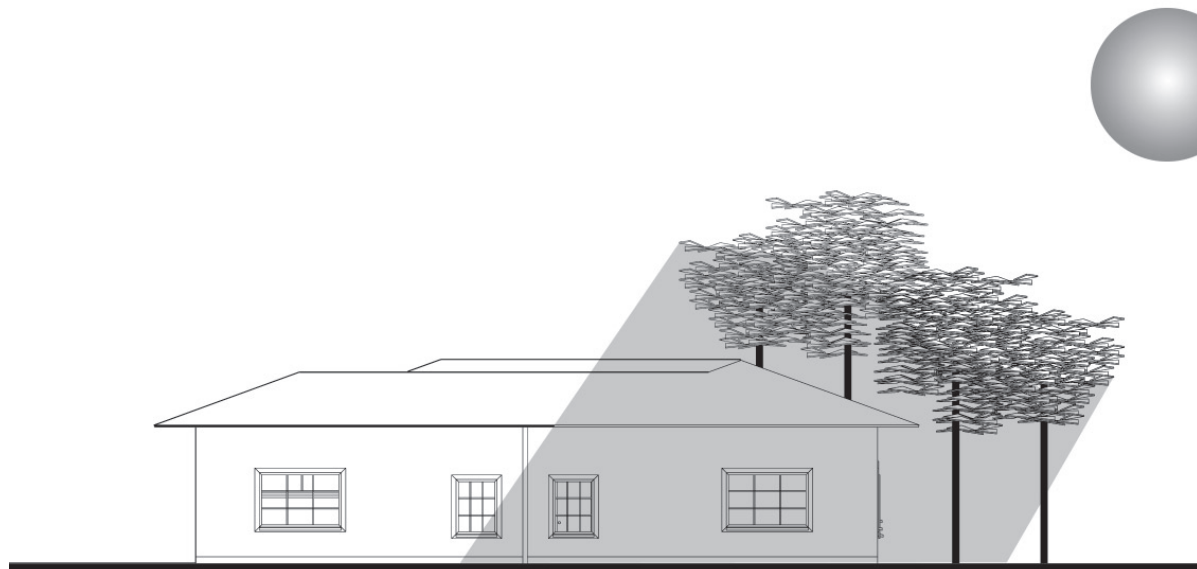
Fig. 8-1: Preventing Heat Gain by Shading the Roof.
