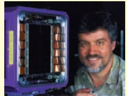
Dr. Gerard Luppino with the 8,192-by-12,288-pixel camera built for the Canada-France-Hawaii Telescope . The focal plane measures 12 cm x 18 cm and contains twelve CCDs in a 2 by 6 pattern.
