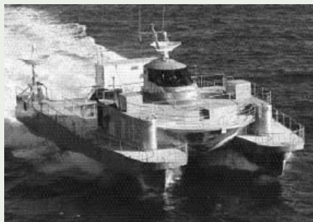
Hawaii's high-tech engineering is embodied in this twin-hulled SLICE vessel. Pacific Marine
