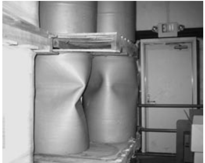
Unsafe storage practices can lead to dangerous situations! These plastic containers of 2,4-D were stacked too high and could have resulted in a spill or injury.
