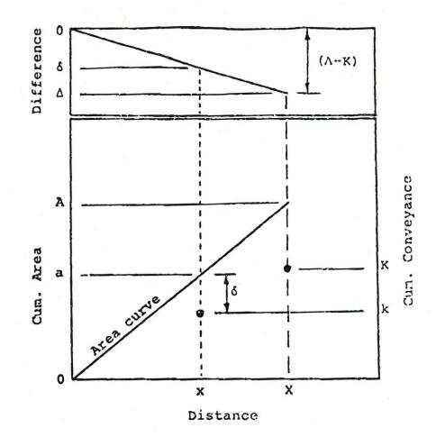
Hence, X is plotted at a distance  $\alpha$ X inches from the origin, A at  $\beta$ A inches from origin, and K at  $\gamma$ K inches from origin.
