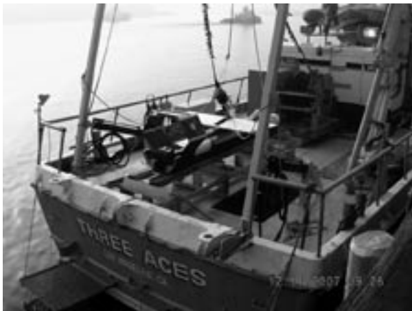
Figure 5. Test vessel Three Aces with long-range side scan sonar in Los Angeles Harbor. Photo by Michael Webb, NOAA.
