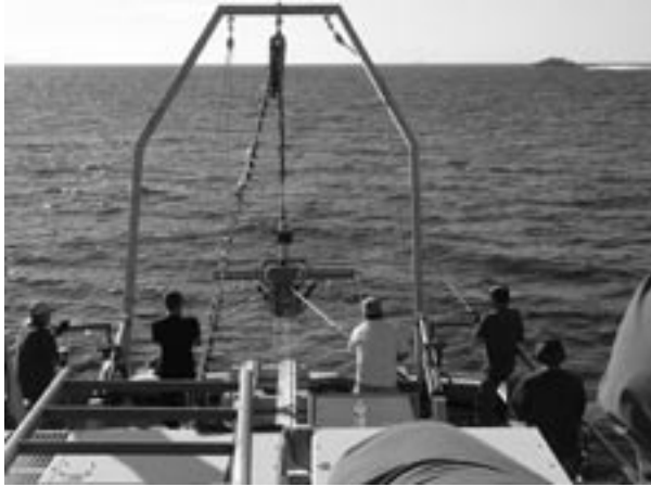
Figure 4. Launching the long-range side scan sonar from the test vessel Three Aces off Catalina Island, California. Photo by Bob McConnaughey.
