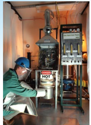
Lead bismuth is being tested in connection with the Lead-Cooled Fast reactor, one of six Gen IV reactor systems concepts.
