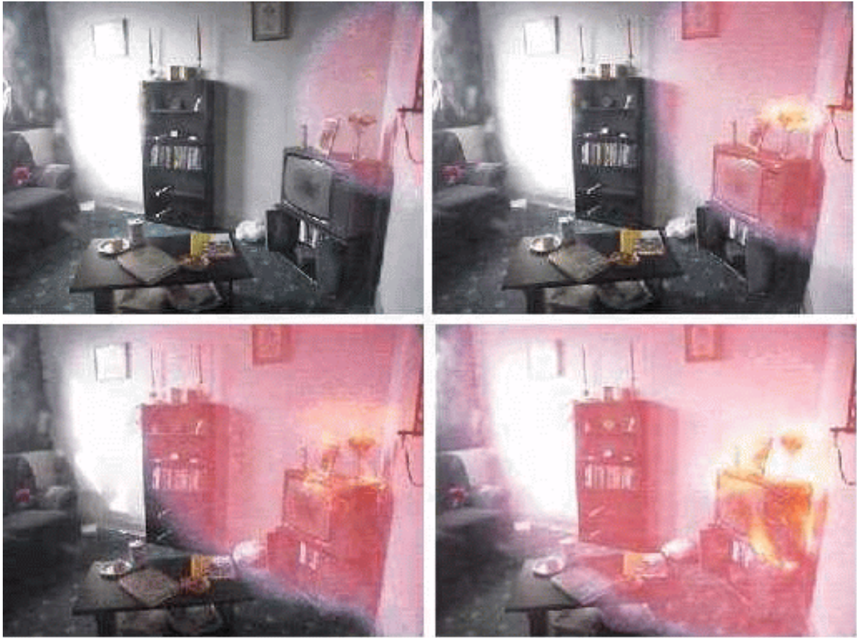
Figure 5. A methane gas explosion propagates through a living room. Experiment conducted by BRE's Fire Research Station for Fire Investigators at the BRE Cardington Laboratory (UK).
