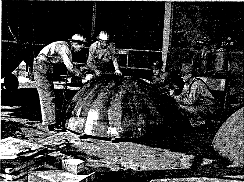
Leadburners fabricating sulphuric acid vat. O. F. Manuel, H. Wright, T. E. Rush, and J. W. South (1951). ▼
