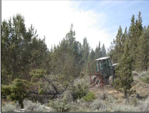
The tractor mounted saw (above) can treat one to three acres per hour in this and similar juniper stands. The gas powered brush cutter (right) is effective in controlling young trees.
