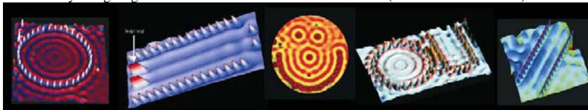
Fig. 5. Left to right: Circular quantum corral, molecular shooting range, atomic smiley, OU atomic logo, and an atomic fence. The atomic smiley and OU logo are used for the nanoscience outreach.
