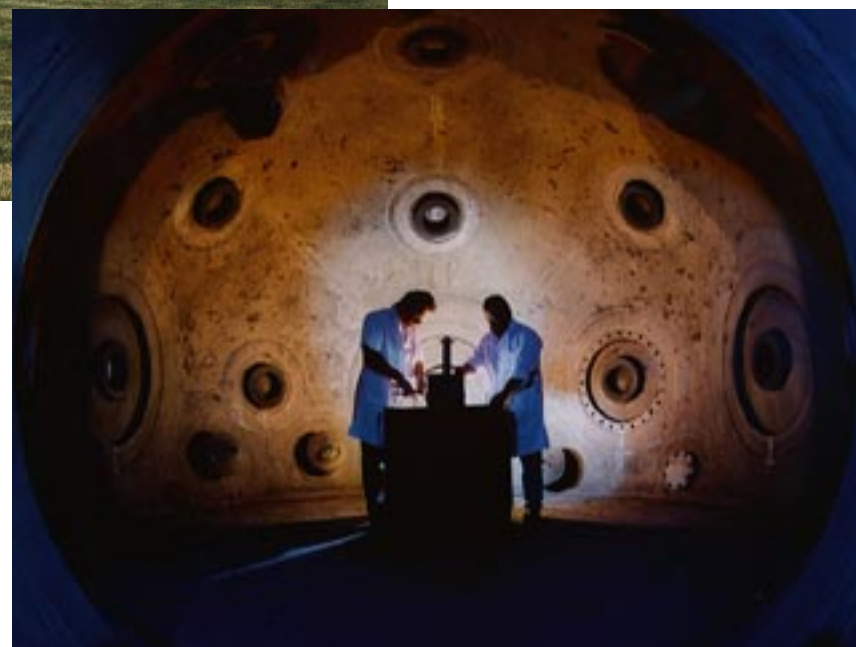
Figure 1. (above) Livermore’s High Explosives Applications Facility (HEAF), completed in 1989, is playing a major role in developing and characterizing high explosives. (right) Specially designed containment vessels are used to safely detonate high explosives in quantities as large as 10 kilograms of TNT-equivalent.
