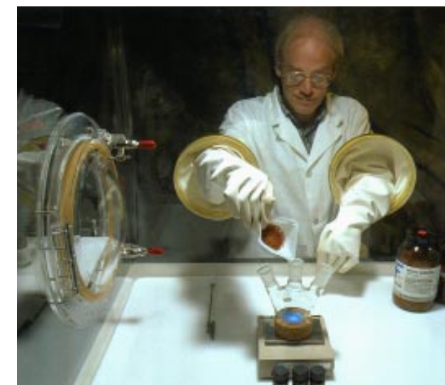
Figure 3. Organic chemist Phil Pagoria synthesizes a new high-energetic compound inside a glovebox to guard against unwanted moisture.
