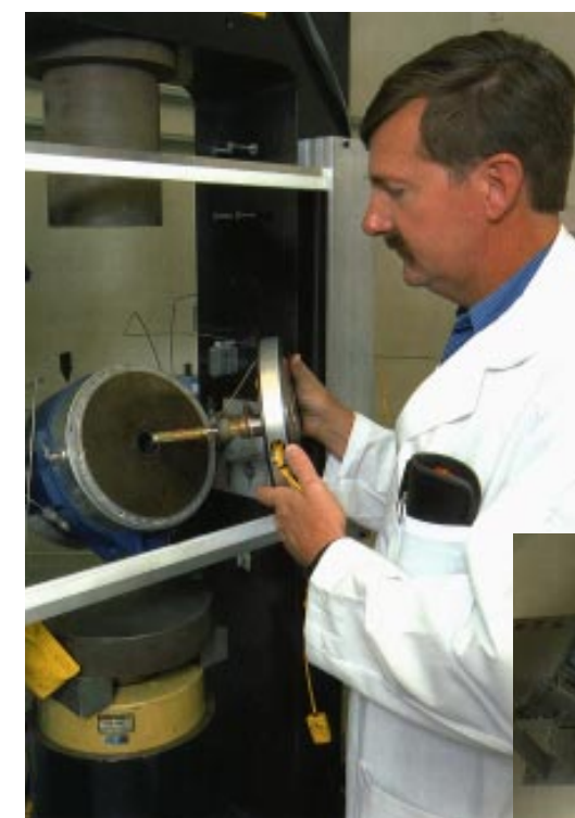
Figure 4. Scientific Associate Chet Lee measures the burn rate of a high explosive under high pressure, a standard safety test.
