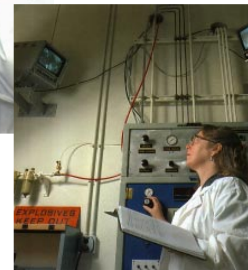
Figure 5. Chemist Rosalind Swansiger remotely controls a performance test of a promising high explosive.
