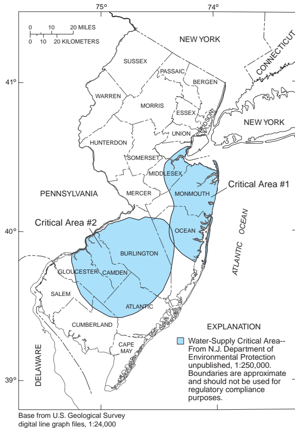
Figure 2. Location of Water-Supply Critical Areas in New Jersey. These areas were designated to help control the decline in water levels in some of the confined aquifers. (From Watt, 2000)
