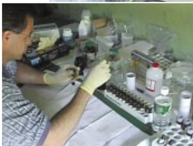
Figure 2. Livermore’s Jeff Haas sampled over 1,200 mortars in two days using the center’s unique thin-layer chromatography screening system.
