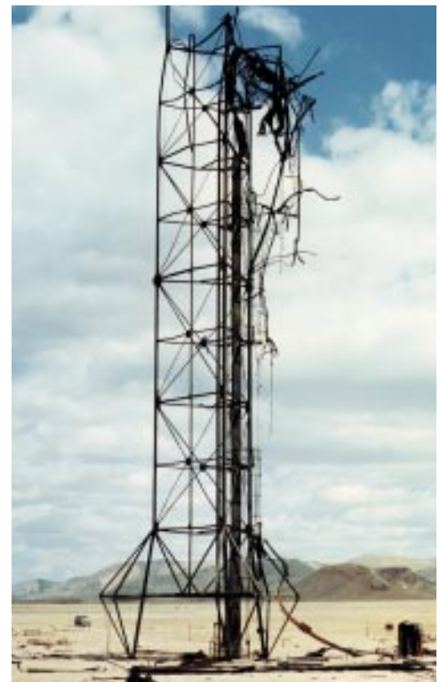
Figure 3. Livermore bomb designers failed their first test. At the Nevada Test Site in 1953, a risky design fizzled, yielding this widely displayed photo of a bent tower.
