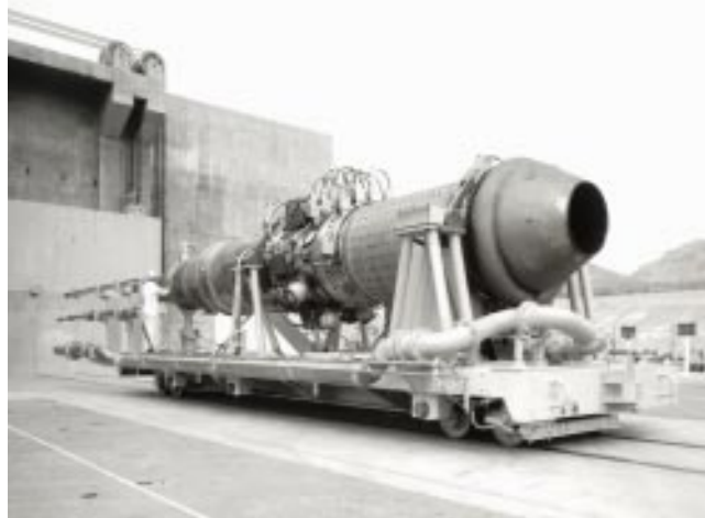
Figure 5. Project Pluto aimed at developing a ramjet engine for the Air Force. Tory II-C, depicted here, was a prototype flight engine tested successfully in 1964.
