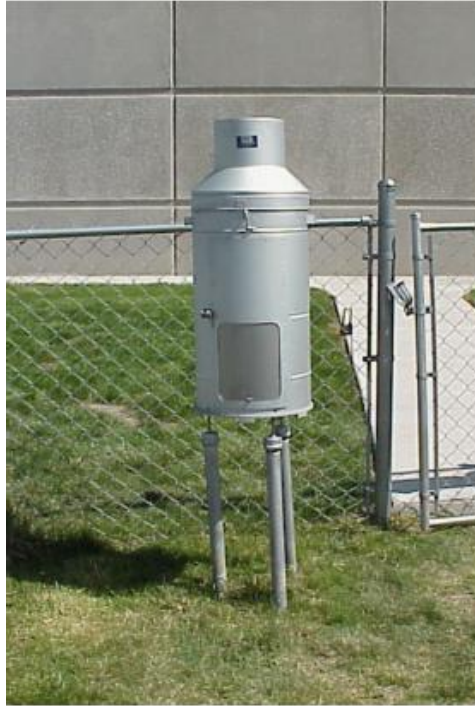
Figure A-9. Universal Weighing Recording Gauge
