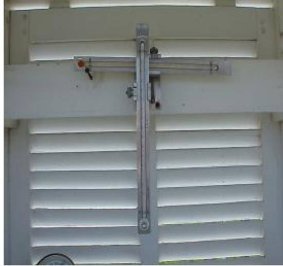
Figure B-9 - Maximum Thermometer in Reading Position
