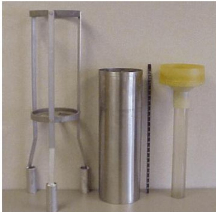
Figure A-4. Eight-Inch Precipitation Gauge Components
