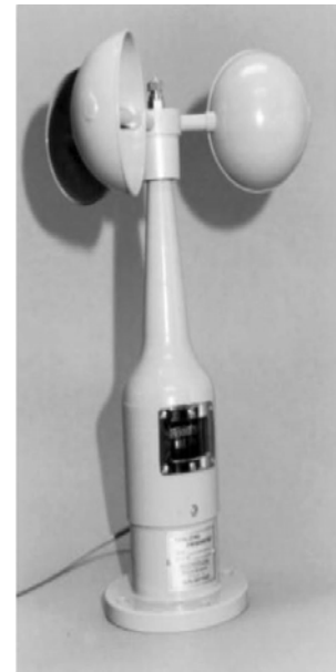
Figure D-8. Totalizing Anemometer with 6 - Digits
