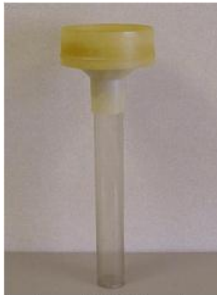
Figure A-31. Measuring Tube with Funnel on Top
