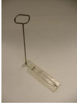
Figure D-13 Submerged Mount Thermometer
