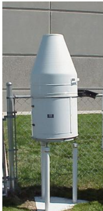
Figure A-10. Fischer & Porter Recording Gauge
