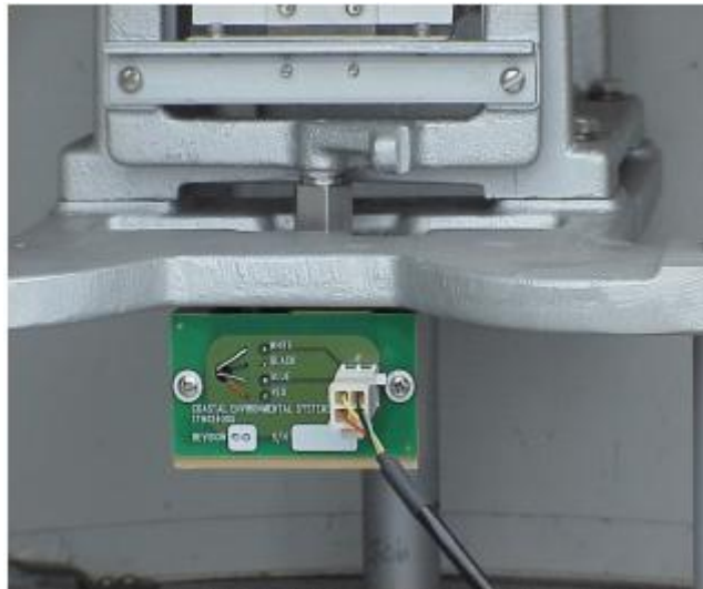
Figure A-15. FPU Front View of Load Cell
