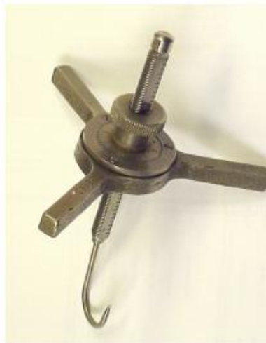
Figure D-6. Hook Gauge
