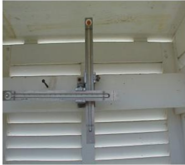
Figure B-11 - Minimum Thermometer in Vertical Position During Resetting of Index
