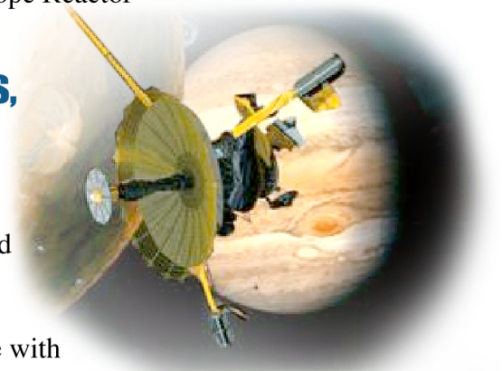
Spacecraft Galileo powered by ^{238}\text{Pu}
