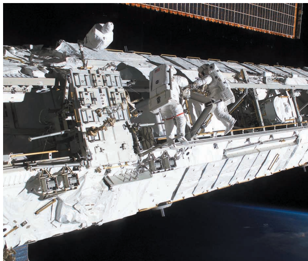
Figure 29: Astronauts John Herrington and Michael Lopez-Allegria work on the newly installed Port-1 truss on the ISS.
