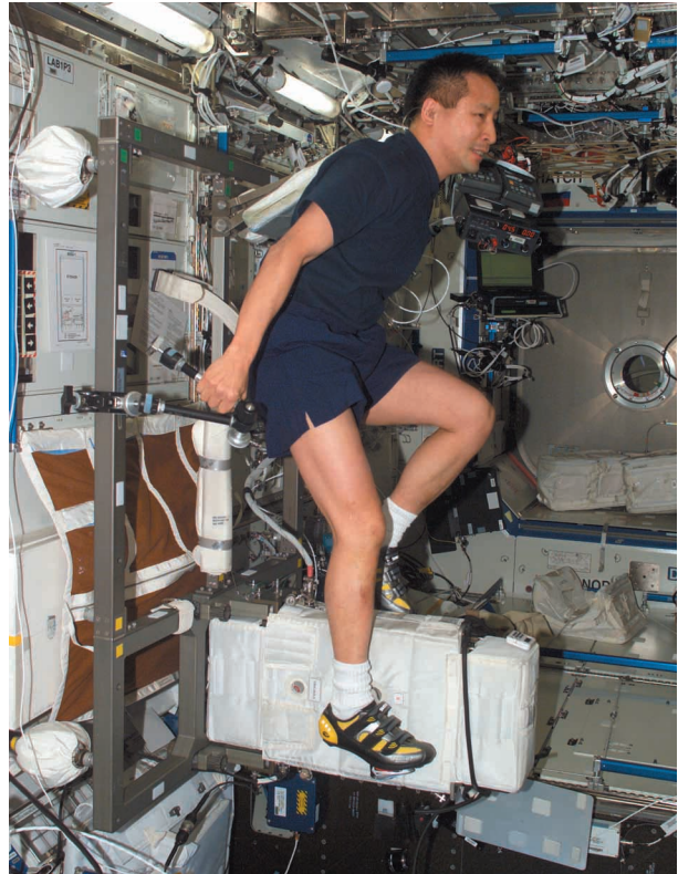
Figure 33: Astronaut Edward Lu exercises on the Cycle Ergometer with Vibration Isolation System (CEVIS) on the ISS.
