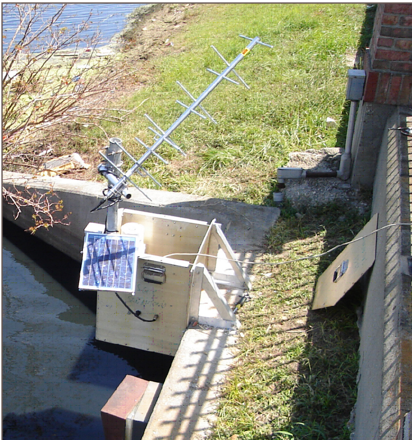
Data from all USGS streamgages, both mobile and permanent, are transmitted by satellite telemetry in real time to the USGS National Water Information System ( http://waterdata.usgs.gov/nwis/rt ).
