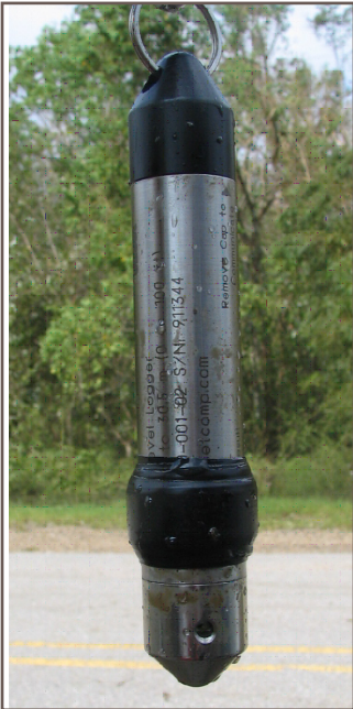
This is the sensor used to collect water-level and barometric-pressure data
