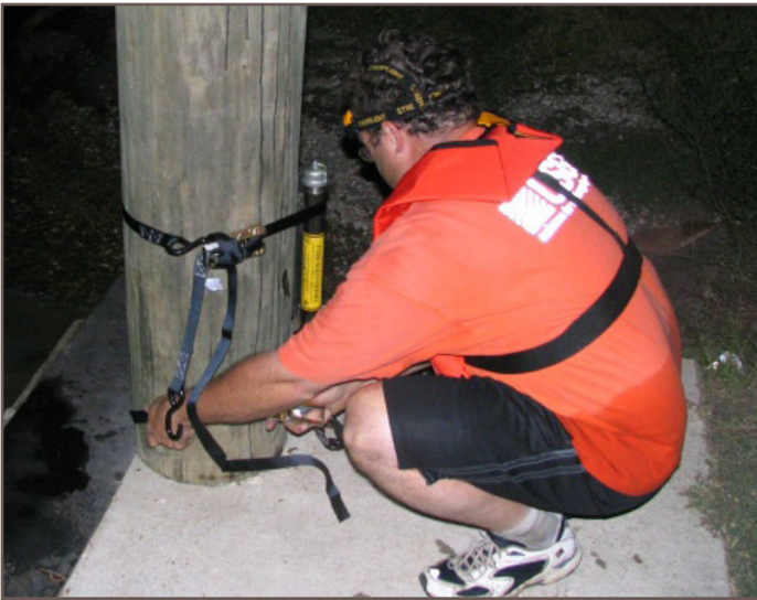
This USGS hydrographer is deploying a storm-surge sensor (in a protective metal casing) to a bridge piling.
