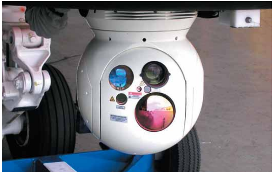
A close-up view showing the FLIR Systems, Inc. Star SAFIRE III electro-optical sensor turret that is to be mounted aboard Coast Guard MH-60T and MH-65C helicopters. The system includes infrared and daylight cameras, laser range finder, and a laser illuminator. U.S. Coast Guard photo
