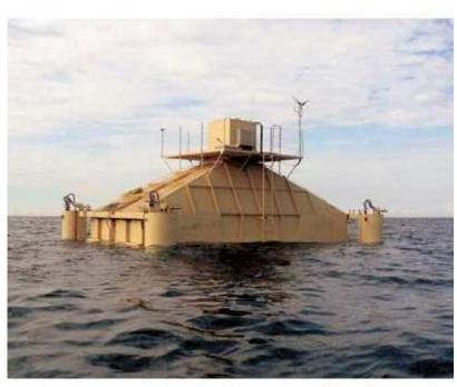
A one-third scale prototype of the 1-megawatt wave generator designed by Oceanlinx Ltd. floats off New South Wales, Australia.
