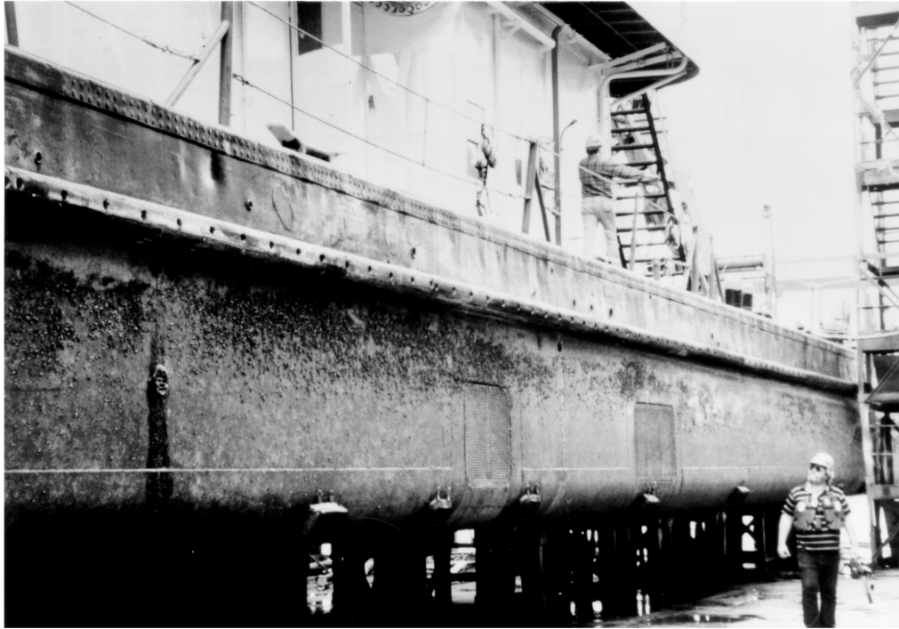
Figure 15. Floating plant hull infested with zebra mussels (courtesy Great Lakes Sea Grant)
