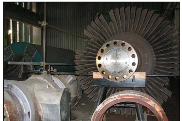
Doura unit 5's damaged low-pressure turbine. Photo: USAID
