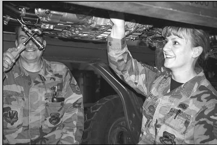
Jet Engine Mechanics Master Sgt. Michael Warrens and Tech. Sgts. Dave Kleinshmit and Karen Smith remove a unified fuel control from an aircraft engine.
